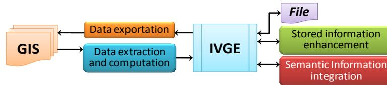
**Figure 1:** Global architecture for IVGE management: in blue, GIS data extraction and associated processes; in orange, IVGE data exportation to GIS format; in green, optional stages for IVGE information enhancement; in red, the semantic information representation using the CG formalism.
