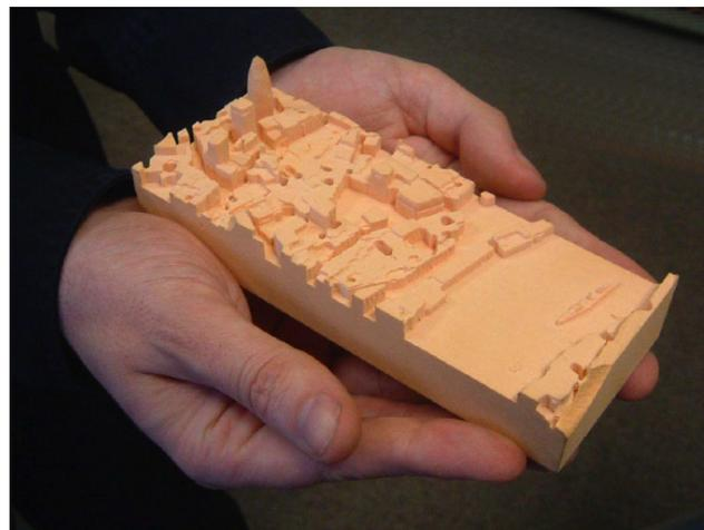
**Figure 2:** 3D architects block model portraying part of central London.
