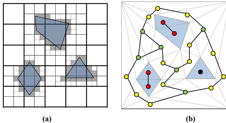
**Figure 3:** Abstraction examples for two kinds of environment descriptions; (a) Grid abstraction using a three levels *quadtree*. (b) Left: topological graph representation of a CDT. Top right: arbitrary abstraction example of this graph.
