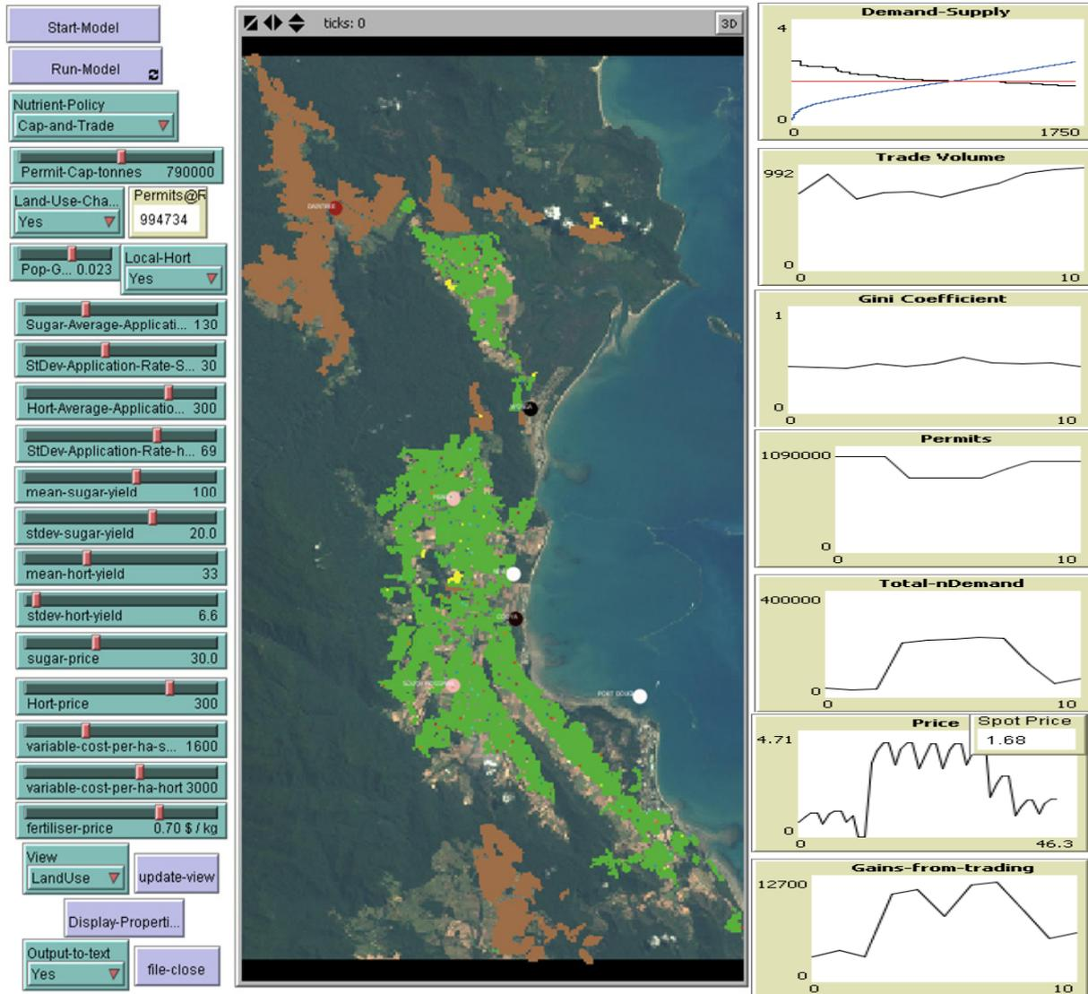
**Figure 7:** Interface for geosimulation of water quality cap-and-trade model testing the effect of land use conversion on market dynamics.
