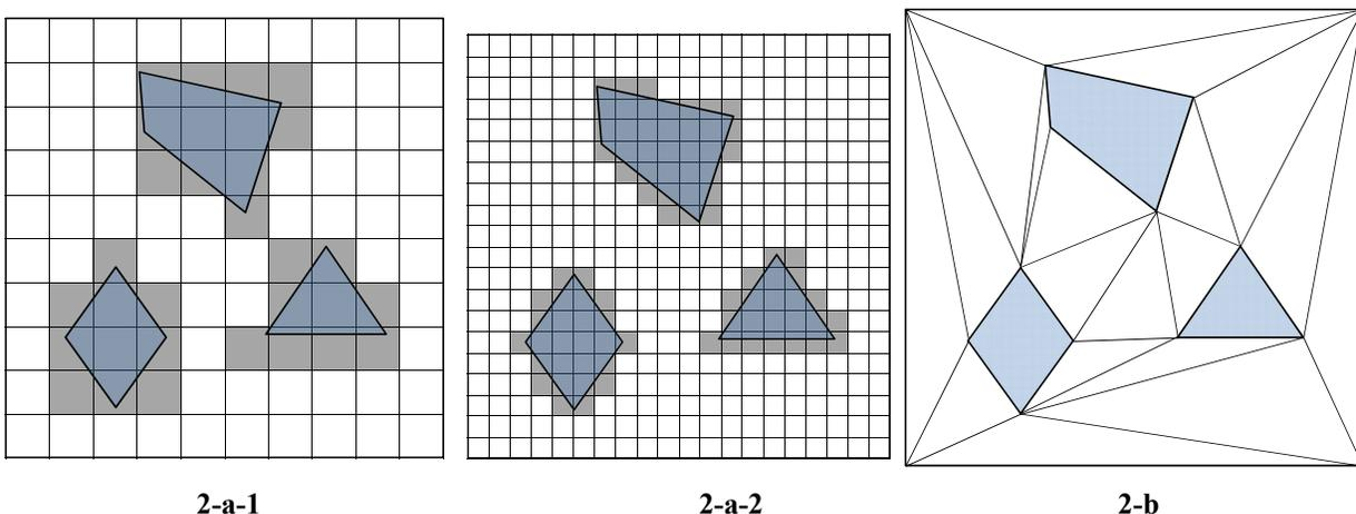
**Figure 2:** Two common cell decomposition techniques; (a) approximate decomposition by grids considering two resolutions; (b) exact decomposition using CDT. White boxes are free, grey are obstacles.
